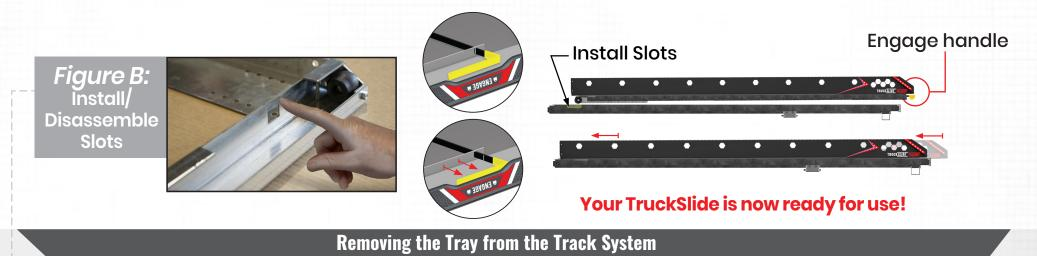
Follow the steps A–C listed below to remove the TruckSlide tray from the rail track system.
